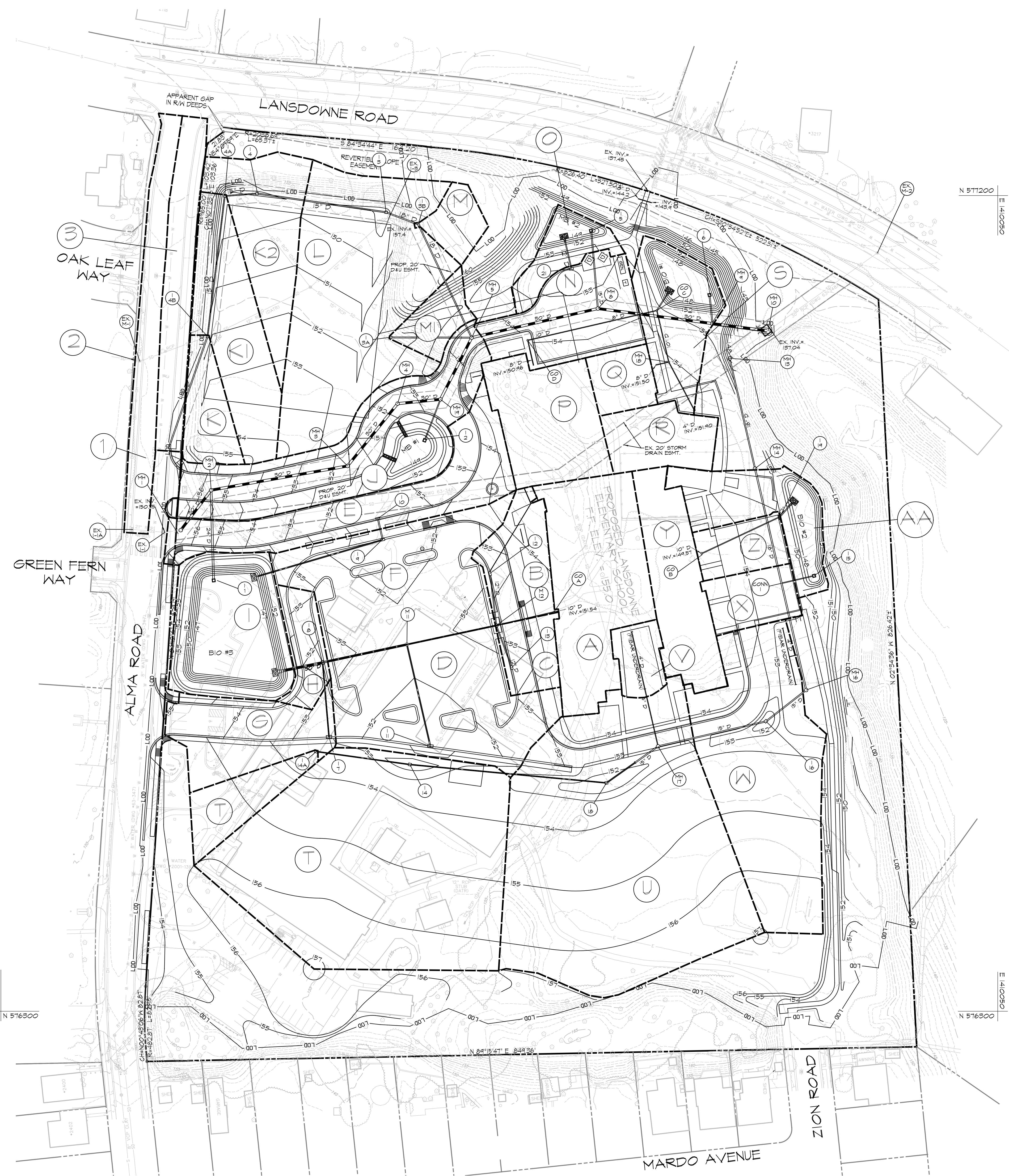
STORM DRAIN DRAINAGE AREA MAP SCALE: 1" = 50'
