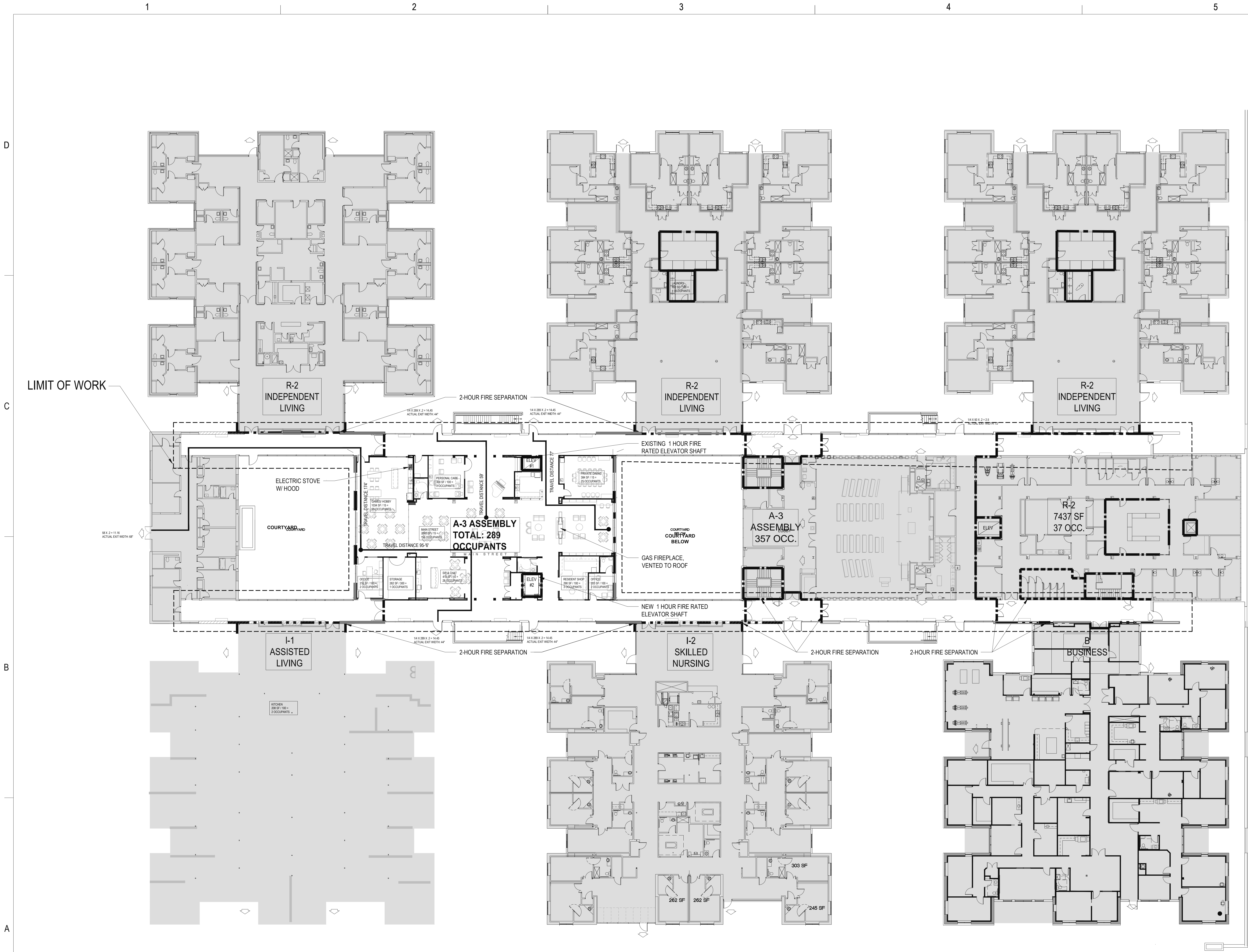
A1 FIRST FLOOR FIRE PROTECTION PLAN SCALE: 1/16" = 1'-0"
