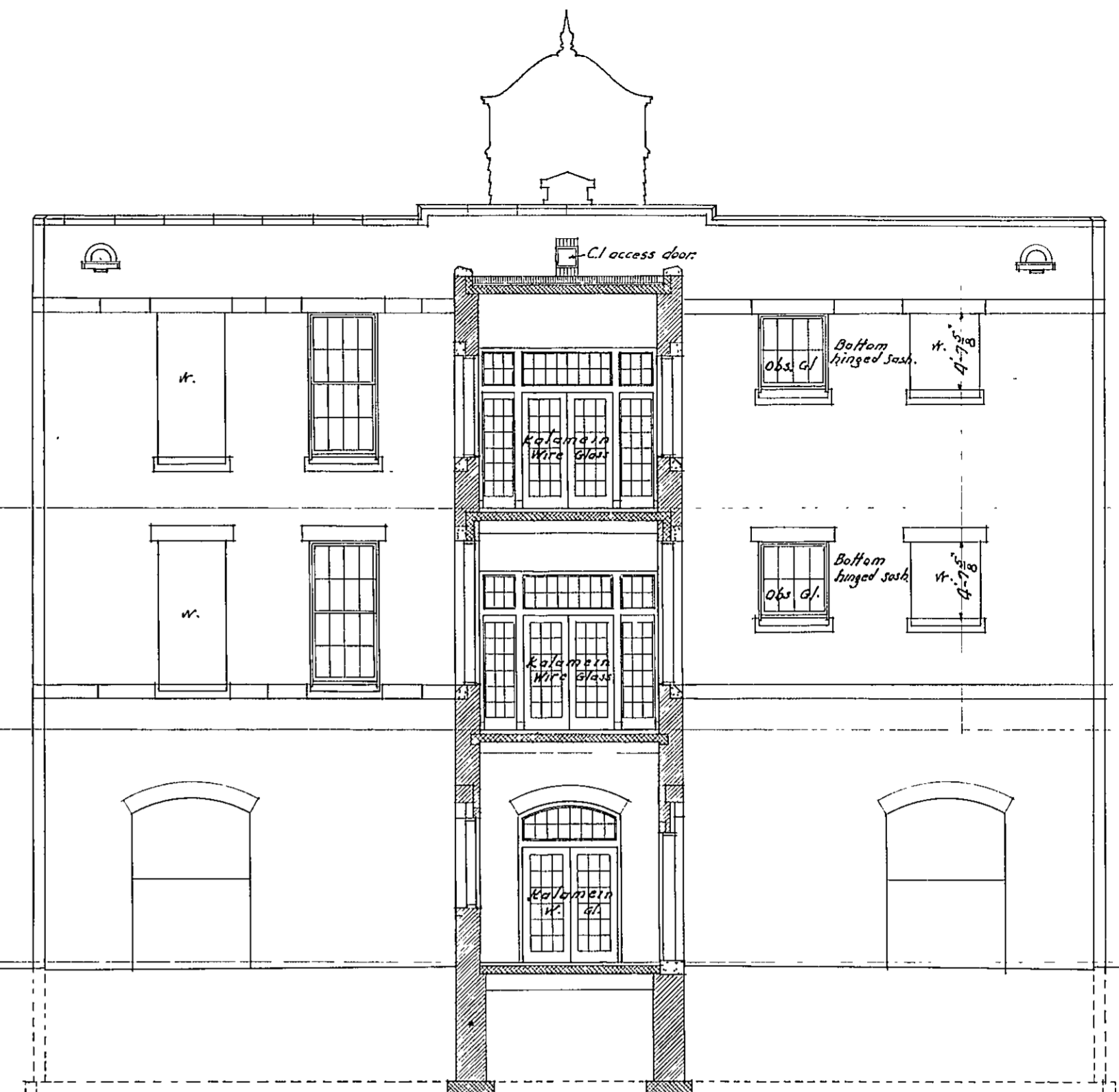
~ SOUTH ELEVATION ~ - SECTION THROUGH SOUTH STAIR HALL -
