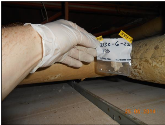
Photograph 31 1" Fitting (TSI3), Room 25, Positive 2% Amosite
