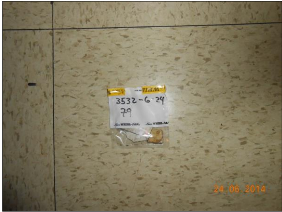
Photograph 18 Floor Tile (FT1), Room 9, Positive 2% Chrysotile Floor Tile Mastic (FT1), Room 9, Positive 2% Chrysotile
