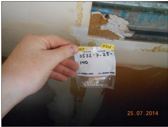
Photograph 34 Joint Compound (DW/JC1), Room 48, Positive 2% Chrysotile
