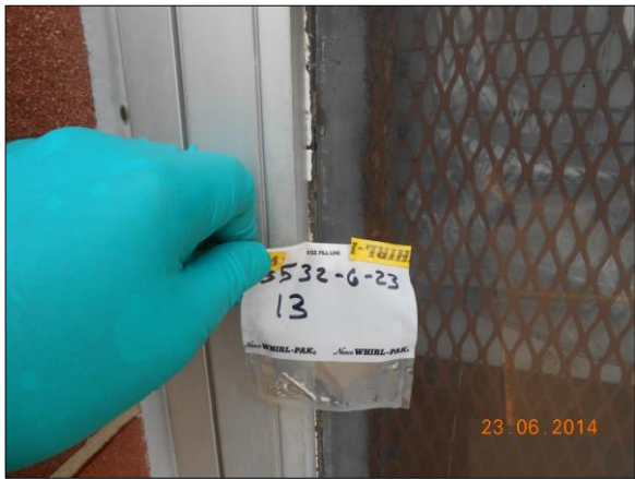
Photograph 15 Window Glaze (OM19), Exterior of Dorm Building, Positive 2% Chrysotile
