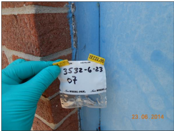
Photograph 9 Door Caulk (OM10), Exterior of SUI Building, Positive 2% Chrysotile
