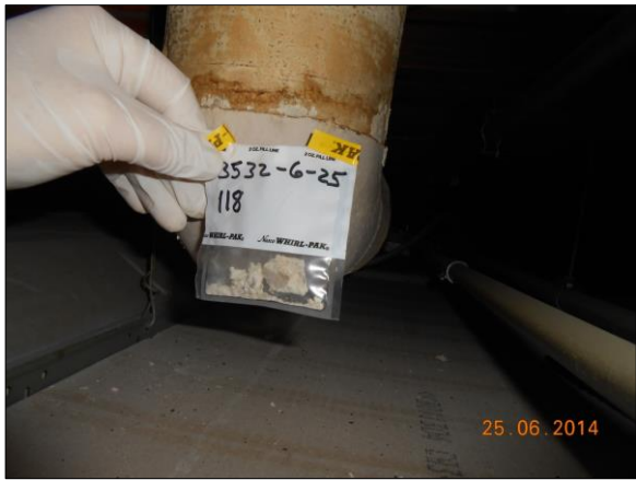
Photograph 30 6" Fitting (TSI2), Room 13, Positive 2% Amosite
