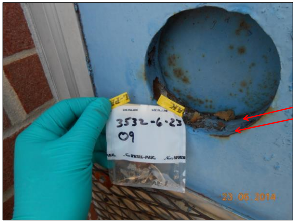
Photograph 14 Window Insert (OM17), Exterior of Dorm Building, Positive 15% Chrysotile
