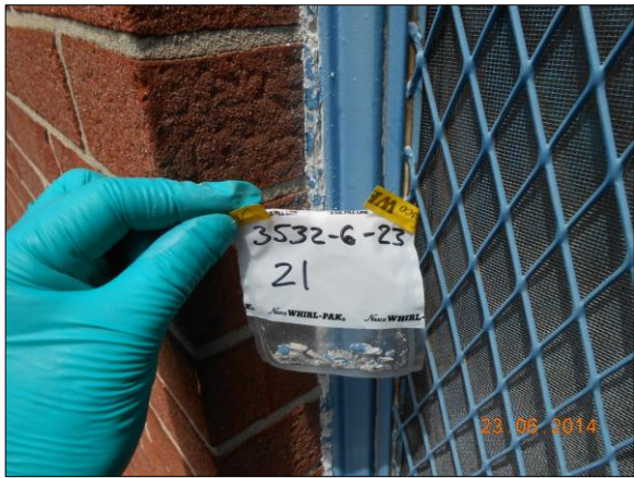
Photograph 10 Window Caulk (OM11), Exterior of SUI Building, Positive 2% Chrysotile
